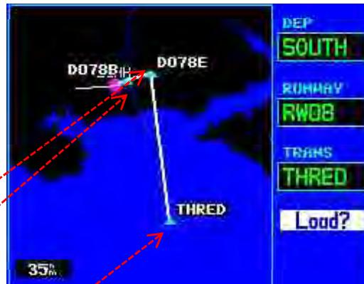
The South departure is coded because it has a specific route (to THRED) and "South" is used as the database identifier even though there is no ICAO identifier. The West departure is not coded, since it lacks a specific route.
