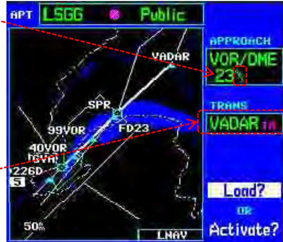
There is no "T crossbar" at the start of this procedure (in part, due to terrain) and SPR is not an IAF. All the IAFs for the procedure are on the STAR charts. VADAR is an example.
