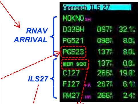
The “man seq” leg name shows that waypoint sequencing is suspended for the Radar Vectoring segment, it is re-engaged in the Garmin 430/530 by pressing the OBS key
