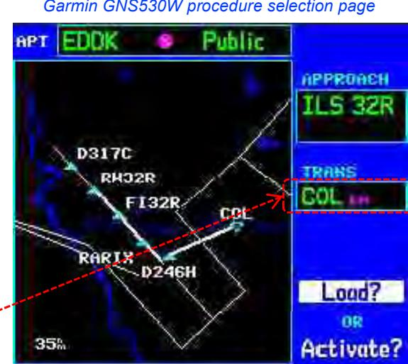
A CNF is created in the coded procedure corresponding to the intersection between the COL 246 radial and the lead-in radial for the turn to the final approach (131 radial KBO)
