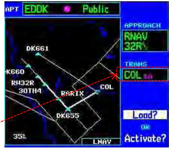
This is not a standard "T" shaped GPS approach, instead the IAFs correspond to the arrival route structure at EDDK
